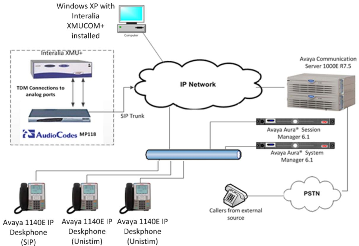
**Figure 1: Network Topology and Connectivity for Interalia XMU+ and Avaya CS1000E**
