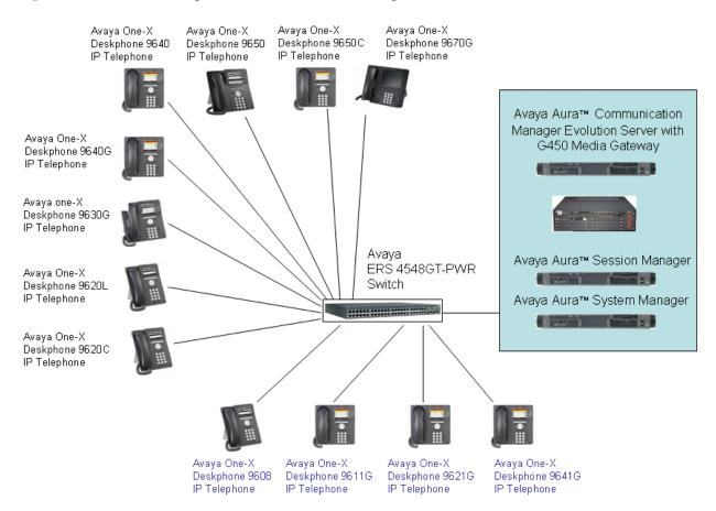
Figure 1 shows the configuration used for PoE testing.
