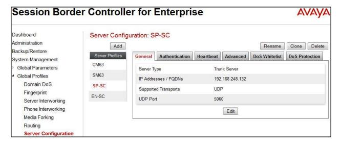
Under **Advanced** tab, check on **Enable DoS Protection**. From the **Interworking Profile** drop down list, select *SP-SC* as defined in **Section 6.2.4**. For **Signaling Manipulation Script**, select *None*. This configuration applies the specific SIP profile to the Frontier traffic. The other settings are kept as default.
