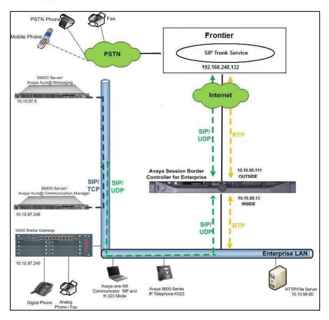
Figure 1: Avaya IP Telephony Network connecting to Frontier SIP Trunking Service
