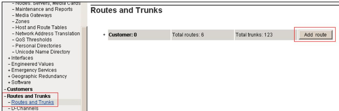
The figure below shows the configuration of the route being added. The values that are boxed in red are to be configured by the user. The values shown are examples used during the solution testing.
