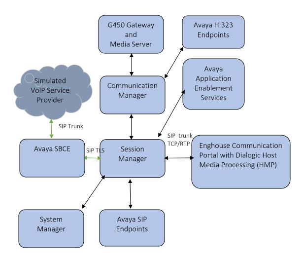
Figure 1: Test Configuration for Enghouse Communications Portal using Dialogic Host Media Processing (HMP) and the Avaya Platform.
