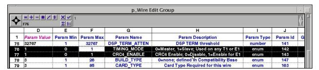
Scroll down the screen as necessary to locate the entry with **Param Id** of "327". Double click on the corresponding **Param Value** field, and enter "1" to enable Alliance to send tones.
