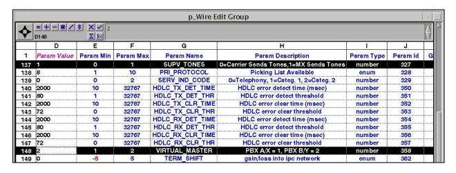
Scroll down the screen as necessary to locate entries with **Param Id** of "364-374" and "603-604". Double click on the corresponding **Param Value** field, and set the values as shown below.
