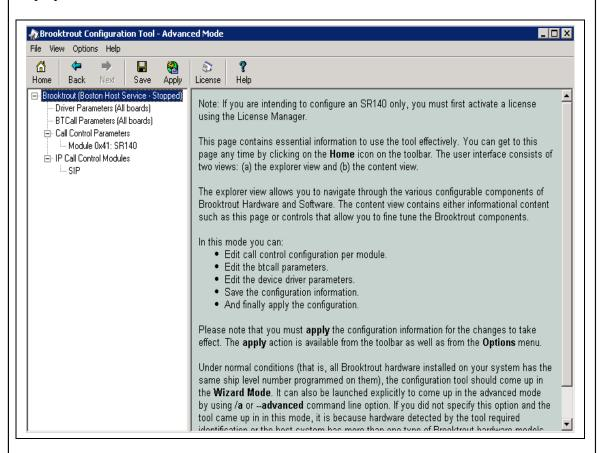
Note that IP Stack can be viewed/reconfigured from the Brooktrout Configuration Tool menu **Options**  $\rightarrow$  **Configure IP Stack**.
