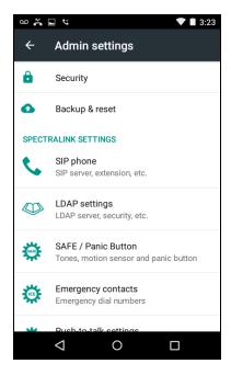
In the subsequent screen shown below, enable the **SIP phone state** by turning the button green, and then click on **Registration 1** to access the SIP parameters.
