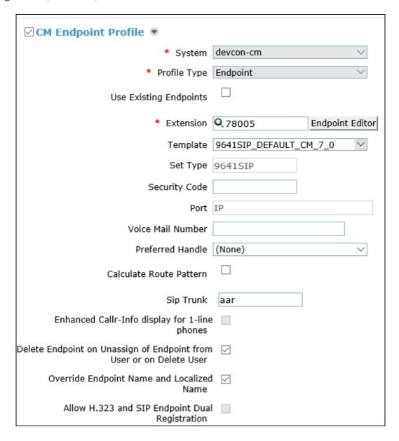
In the **CM Endpoint Profile** sub-section, click the **Endpoint Editor** button to display the page below. In the **General Options** tab, specify that coverage path that points to the voicemail system in the **Coverage Path 1** field. This provides voicemail coverage for the SIP user. In this example, coverage path 10 was used.
