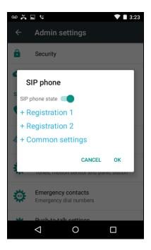
Under the **SIP phone** settings for **Registration 1**, Enter the Session Manager IP address in the **SIP server** field, port 5060 for the **SIP server port** field, UDP for the **Transport** field, and the SIP extension in the **Extension number** field as shown below.
