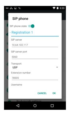
Scroll down the screen to access the other **Registration 1** settings. Enter the SIP extension in the **Username** field, the SIP password in the **Password** field, and the voicemail pilot number in the **Voice mail retrieval address** field. Enable the **Use SIP standard hold signaling** and the **Force subscription to message waiting notifications** options as show below.
