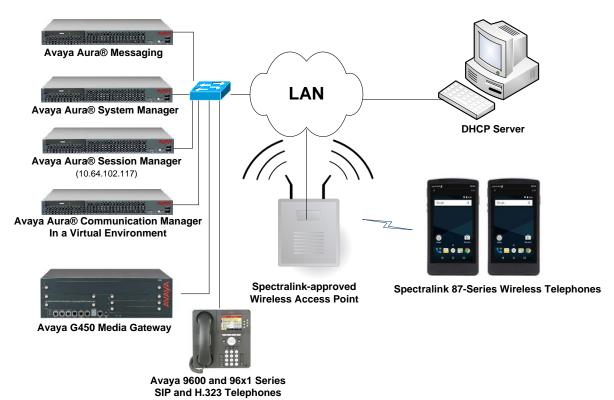
Figure 1: Avaya SIP Network with Spectralink 87-Series Wireless Telephones
