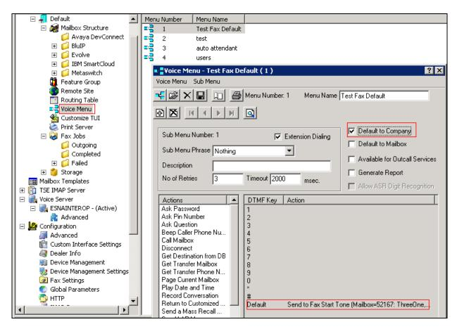
Note: This configuration was used because when a user sends the fax to Officelinx, there is no fax tone sent from Officelinx Server, and the fax on Communication Server 1000 is waiting. As a result, the fax gets no answer. It is necessary to check the "Default to Company" option with Default "Send to Fax start Tone" on Officelinx in order for Officelinx send fax tones to a fax machine.
