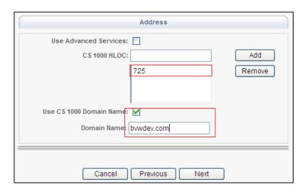
Click **Next** to add Address for CS1K TR87 Service provider. Configure the route address to indicate from where a call is originating.
