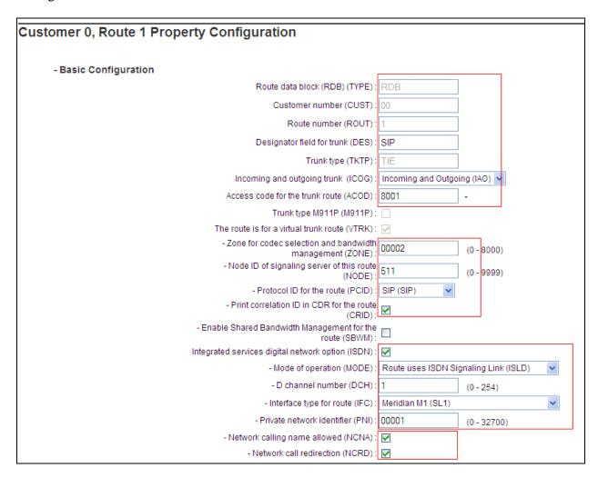
Example of trunk configured during compliance test:
