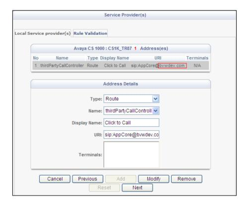
Click **Next** to enter the rule for TR87 Service Provider. Configure simple translation rules to route a web service request to a particular service provider and if necessary, transform the parameters in the request, before presenting them to the service provider.
