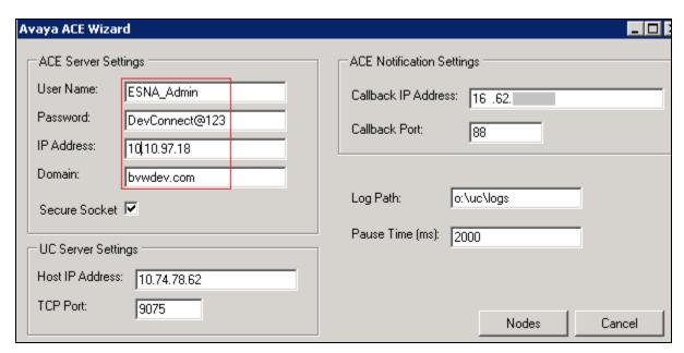
Click on **Nodes** to open the next window where a user manually enters the device extension to get its notification. Click on **Next** button(not shown).
