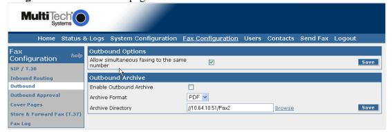
An Outbound approval rule was used to hold outbound faxes for a portion of the testing. This was not a requirement, but was a useful method for traffic test scenarios. The approval setup simply requires a check on the **Enable Outbound Approval** setting, and selecting a **User** to approve outbound faxes:
