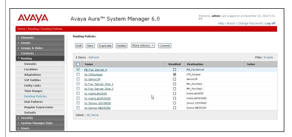
A Routing Policy consists of a definition of the **SIP Entity as Destination**, the **Time of Day** the policy applies, and the **Dial Patterns** that will trigger this particular policy. Below are the settings used for this test. Use the **Select** or **Add** buttons to create or use existing definitions for each parameter.
