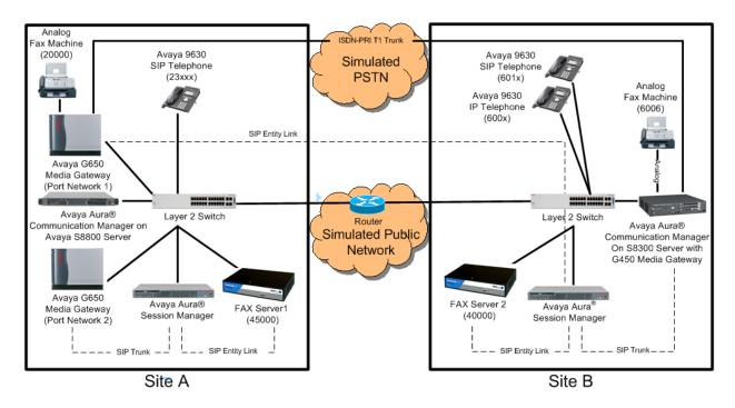
Figure 1: Multi-Tech FaxFinder® IP Fax Server sample configuration
