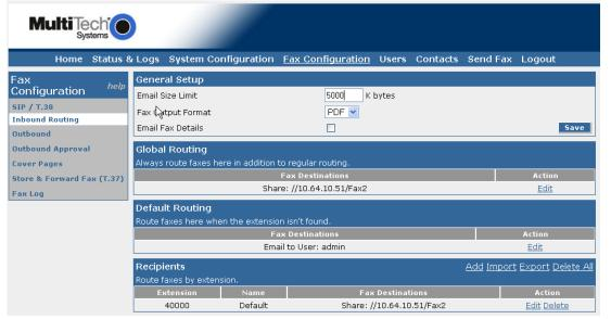
Global Routing was configured by clicking the **Add** link (from the dialog that appears when the **Edit** link is clicked in **Global Routing**), this rule applies to all Faxes received, in addition to any other routing rules:
