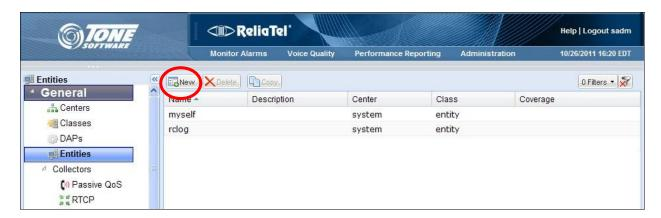
In the lower portion of the screen, select the **General** tab. Enter a descriptive **Name** and a desired **Description** for the MSS. Select the appropriate pre-configured **Center** from the drop-down list, in this case "production". For **Class**, select "cl-avaya-mm".
