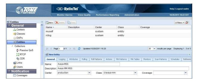
Select the **Logging** tab. Check the **Log State** field. For **Channel**, enter the corresponding channel name from **Section 7.2**. For **Log Pattern**, select "l-amm" from the drop-down list. Retain the default values in the remaining fields.
