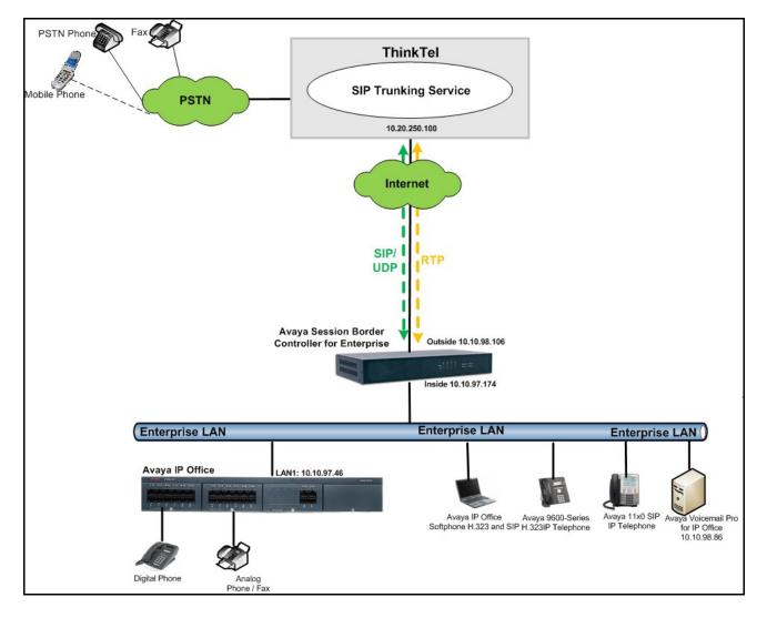
Figure 1: Avaya IP Telephony Network Connecting to ThinkTel SIP Trunking Service.
