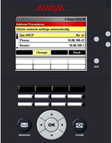
Using the up and down scroll buttons, select the appropriate fields for editing, pressing the **Change** button to edit each field. Scroll down further to see the fields for Mask (subnet mask), HTTPS & HTTP File Server, DNS Server, 802.1Q, VLAN ID, and VLAN Test.
