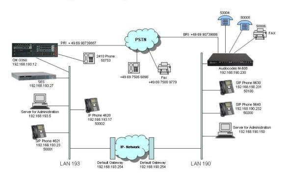
Figure 1 AudioCodes Mediant-600 Test Configuration
