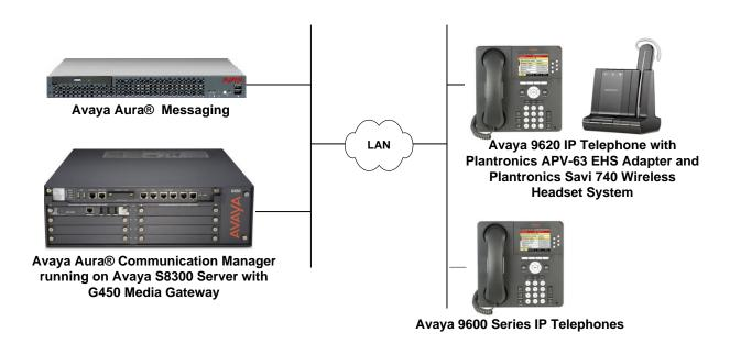
Figure 1: Avaya 9600 Series IP Telephone with Plantronics APV-63 EHS Adapter and Plantronics Savi 740 Wireless Headset System
