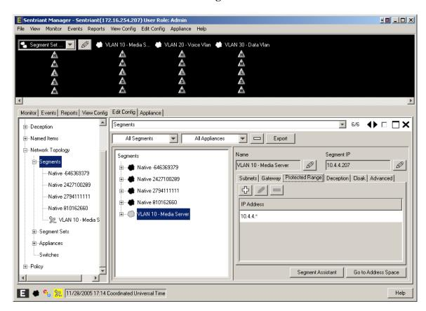
To protect specific ranges within the subnet, uncheck the **Add Protected Rang** checkbox and configure the ranges in the **Protected Range** tab (not described in these Application Notes)
