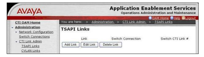
The Add / Edit TSAPI Links screen is displayed next. The Link field is only local to the Application Enablement Services server, and may be set to any available number. For Switch Connection, select the relevant switch connection from the drop-down list. In this case, the existing switch connection "S8500" is selected. For Switch CTI Link Number, select the CTI link number from Section 4.3. Retain the default values in the remaining fields, and click Apply Changes.
