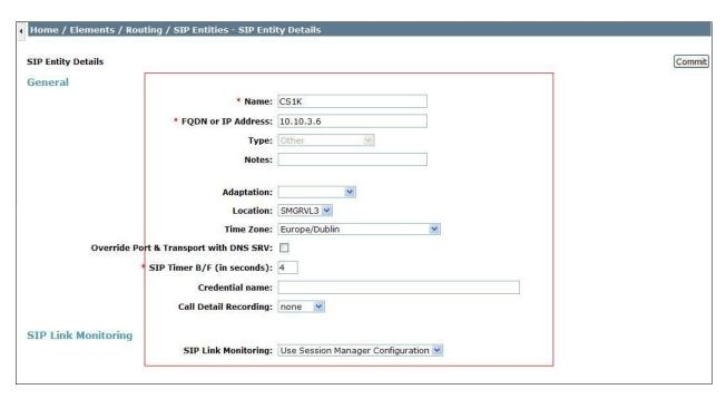
The following screen shows the addition of Avaya SBCE SIP Entity. The **FQDN or IP Address** field is set to the IP address of its private network interface.
