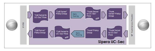
To create a Server Flow, navigate to UC-Sec Control Center → Device Specific Settings → End Point Flows. Select the Server Flows tab and click Add Flow.
