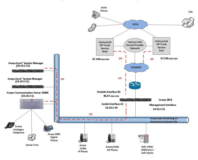
Figure 1: Test Setup CenturyLink SIP Trunk Service to Avaya Enterprise
