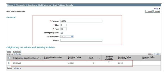
The second example shows that a minimum 5 digit dialed numbers that begin with 00353 originating from SMGRVL3 uses route policy toSipera. This will allow outbound calls to route from the CS1000E to PSTN test numbers in the Avaya enterprise lab.
