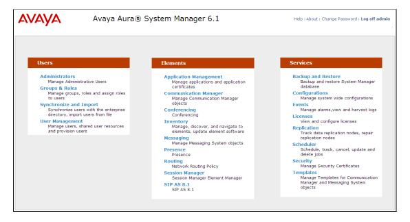
Most of the configuration items are performed in the Routing Element. Click on **Routing** in the Elements column shown above to bring up the Introduction to Network Routing Policy screen.
