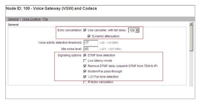
Next, scroll down and configure the **Codec G.711**. The relevant settings are highlighted in the following screenshot.
