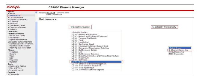
Select **Status for D-Channel (STAT DCH)** command and click **Submit** to verify status of virtual D-Channel as shown below. Verify the status of the following fields.
