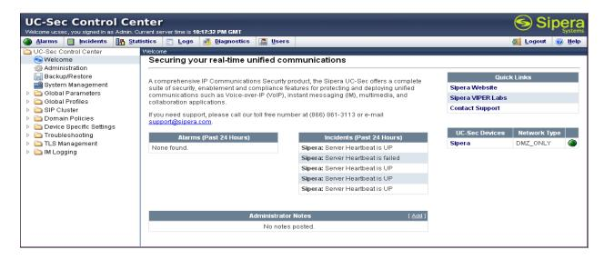
To view system information that was configured during installation, navigate to UC-Sec Control Center → System Management. A list of installed devices is shown in the right pane. In the case of the sample configuration, a single device named Sipera is shown. To view the configuration of this device, click the monitor icon (the third icon from the right).
