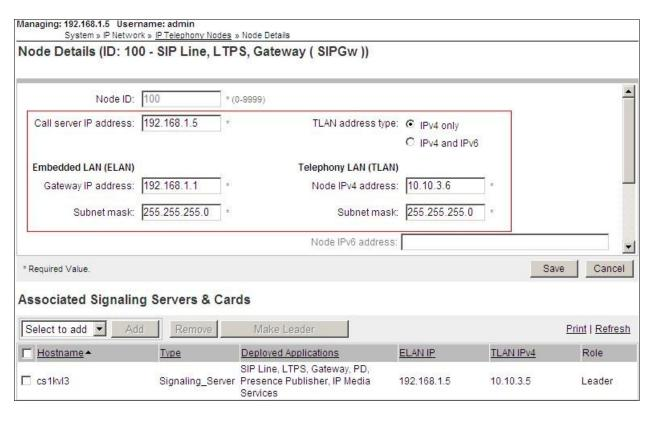
The next screenshots show the SIP Virtual Trunk Gateway configuration, navigate to System → IP Networks → IP Telephony Nodes → Node Details → Gateway (SIPGW) Virtual Trunk Configuration Details and fill in the highlighted areas with the relevant settings.
