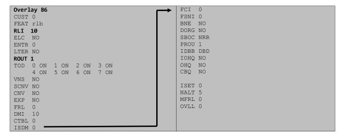
Next, configure Co-ordinated Dialling Plan(s) (CDP) which users will dial to reach PSTN numbers. Use the CS1000E system terminal and **Overlay 87**. The following are some example CDP entries used. The highlighted **RLI** value previously configured in overlay 86 is used as the Route List Index (**RLI**), this is the default PSTN route to the SIP Trunk service.
