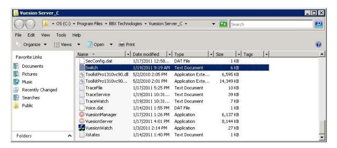
Open the **Switch** text file with the NotePad application. For **SIPPROXYADDRESS**, enter the IP address of IP Office from **Section 5.2**. For **SIPPROXYPORT**, enter the UDP port number from **Section 5.3**. For **SIPMYIPADDRESS**, enter the IP address of the local Ethernet interface used for connectivity with IP Office, in this case "110.10.10.104".
