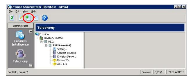
The **Add Contact Source** screen is displayed. Enter a descriptive **Name**. Select "Avaya PDS" as **Contact Source Type**, and click **OK**.
