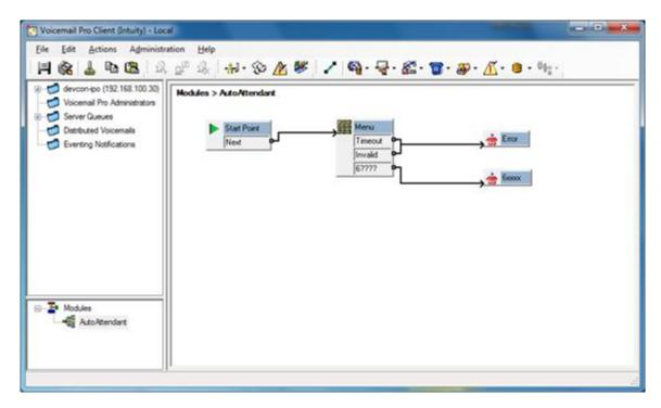
Select File  $\rightarrow$  View As Text from the top menu to view the Voicemail Pro configuration as a text file, which contains the Auto Attendant module and the two recording files. The ViewAsText.txt screen is displayed as shown below. Select File  $\rightarrow$  Save As from the top menu.
