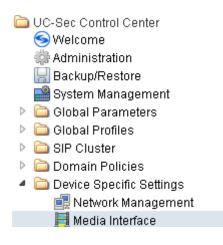
Under UC-Sec Devices, select the device being managed, which was named "Sipera-outside-1112" in the sample configuration (not shown). Select Add Media Interface.
