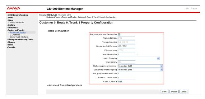
Click on Edit Class of Service, For Media Security, select Media Security Never (MSNV), for Restriction Level enter Unrestricted (UNR). Use default for remaining values. Scroll down to the bottom of the screen and click Return Class of Service and then click on the Save button (not shown).
