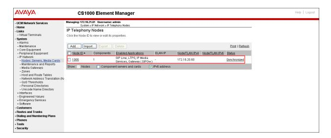
The **Node Details** screen is displayed as shown below with the IP address of the Avaya CS1000 node. The **Node IP Address** is a virtual address which corresponds to the TLAN IP address of the Signaling Server, SIP Signaling Gateway. The SIP Signaling Gateway uses this **Node IP Address** to communicate with other components for call processing.
