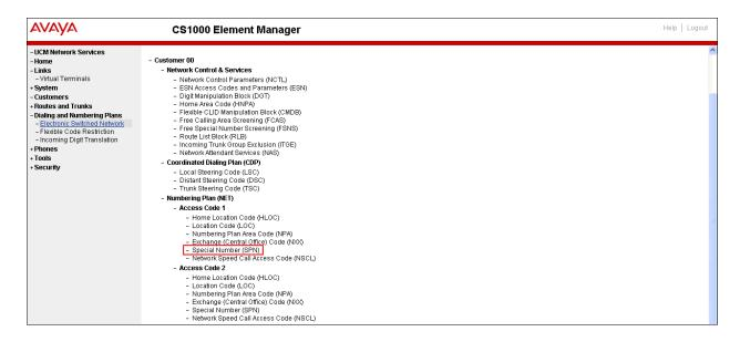
Enter **SPN** and then click on the "**to Add**" button. Examples of special numbers that were used for the testing are shown below.
