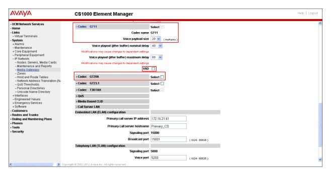
Currently for Fax over IP, CenturyLink does not support **T.38**, only **G.711u pass-through**. G.711 was chosen as default codec. Ensure that **Enable V.21 FAX tone detection** is unchecked, and that **Enable modem fax pass through mode** is checked. This configuration enables **G.711** pass through codec for fax.
