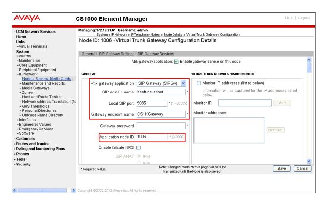
Click on the **SIP Gateway Settings** tab, under **Proxy or Redirect Server**, enter the following values (highlighted in red boxes) for the specified fields, and retain the default values for the remaining fields as shown below.
