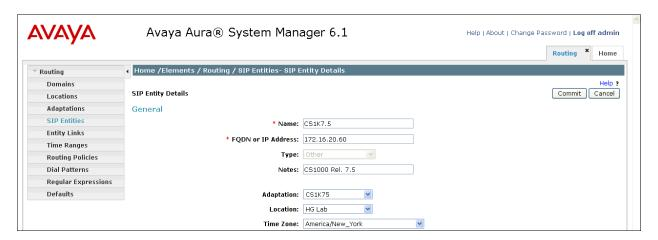
The following screen shows the addition of the Acme SBC SIP entity.
