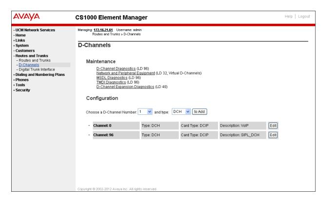
The D-Channels 0 Property Configuration screen is displayed next as shown below (D-Channel 0 was added for the testing). Enter the following values for the specified fields:
