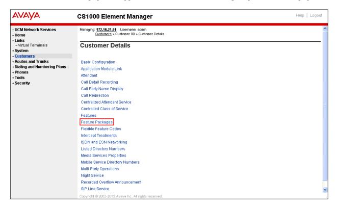
The screen is updated with a list of Feature Packages populated. Select Integrated Services Digital Network to edit its parameters. The screen is updated with parameters populated below Integrated Services Digital Network. Check the Integrated Services Digital Network (ISDN) checkbox, and retain the default values for all remaining fields as shown below. Scroll down to the bottom of the screen, and click on the Save button at the bottom of the page.
