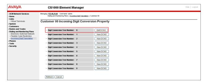
Detail configuration of the **DCNO** is shown below. The **Incoming Digits** can be added to map to the **Converted Digits** which would be the Avaya CS1000 system extension number. This **DCNO** has been assigned to route 0 as shown in **Section 5.5.5**.
