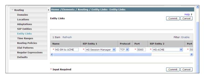
The following screen shows the list of Entity Links. Note that only the highlighted links were created for the compliance test, and are the ones relevant to these Application Notes.
