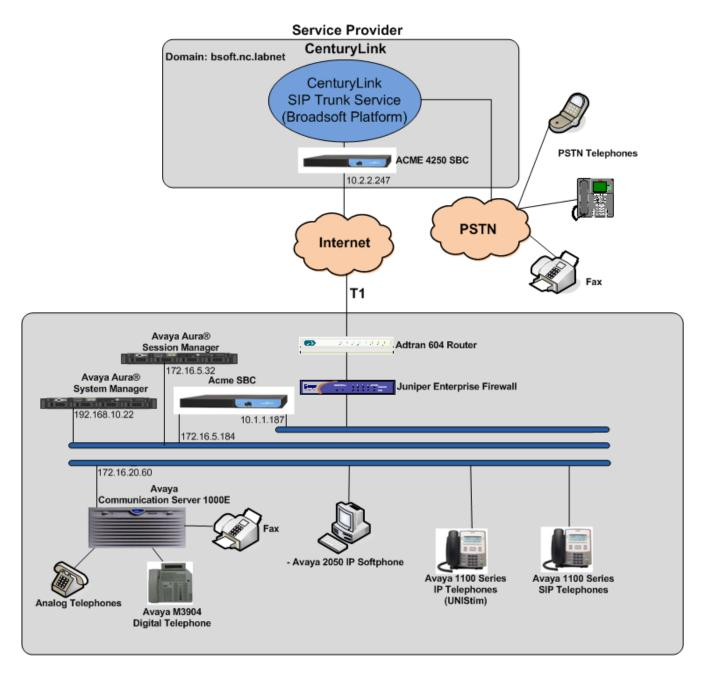
Figure 1: CenturyLink BroadWorks SIP Trunk Service and Avaya CS1000E
