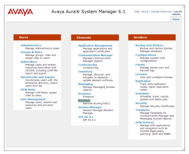
The navigation tree displayed in the left pane below will be referenced in subsequent sections to navigate to items requiring configuration. Most items discussed in this section will be located under the **Routing** link shown below.
