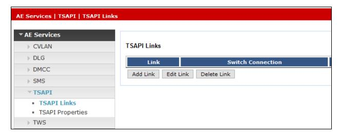
The **Add TSAPI Links** screen is displayed next. The **Link** field is only local to the Application Enablement Services server and may be set to any available number. For **Switch Connection**, select the relevant switch connection from the drop-down list. In this case, the existing switch connection "Duplex" is selected. For **Switch CTI Link Number**, select the CTI link number from **Section 5.2**. Retain the default values in the remaining fields and click **Apply Changes**.
