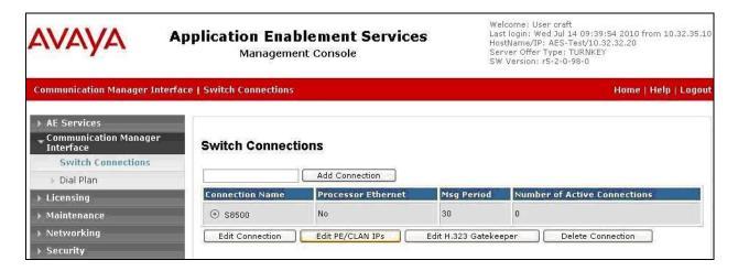
The **Edit H.323 Gatekeeper** screen is displayed. Enter the IP address of a C-LAN circuit pack or the Processor C-LAN on Communication Manager to be used as H.323 gatekeeper, in this case "10.32.32.12" as shown below. Click **Add Name or IP**.
