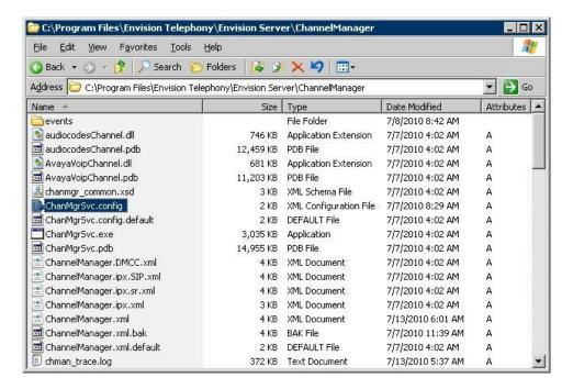
Open the **ChanMgrSvc.config** file with the WordPad application. Enter the following values for the specified fields, and retain the default values for the remaining fields.
