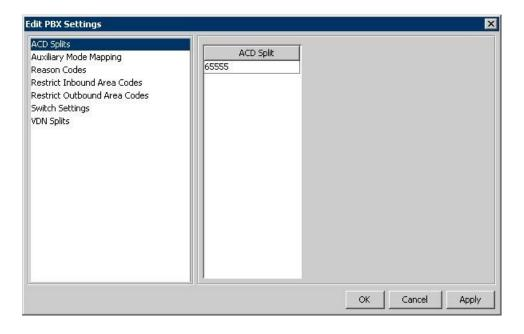
Select **Switch Settings** from the left pane. For **Service Observation Code**, enter a non-blank value. Retain the default values in the remaining fields.
