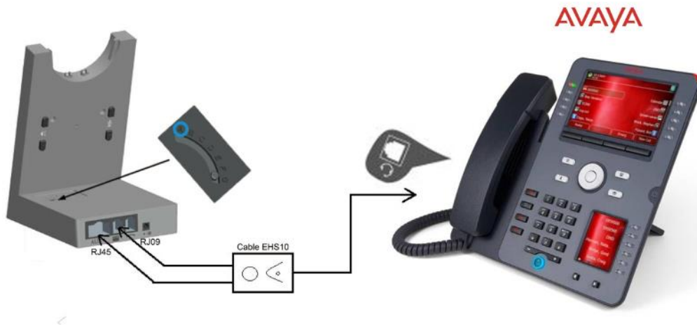
Figure 2: Setup of VT EHS10 cable with VT 9400 DECT headset base to Avaya J100 Series IP Deskphone
