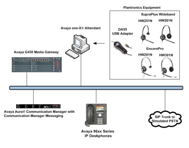
**Figure 1: Test Configuration**
