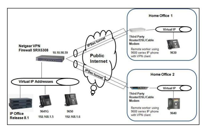
Figure 1: Remote User Home Office Connecting via IPSec tunnel (established by Netgear VPN) to IP Office Configuration
