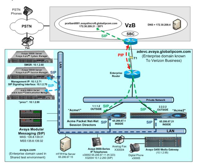
Figure 1: Avaya Interoperability Test Lab Configuration
