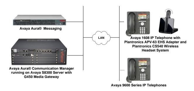
Figure 1: Avaya 1600 Series IP Telephone with Plantronics APV-63 EHS Adapter and Plantronics CS540 Wireless Headset System
