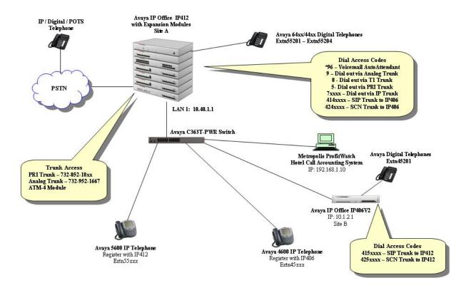
Figure 1. Test configuration of ProfitWatch with Avaya IP Office
