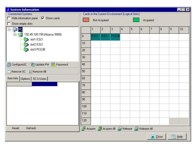
Next, verify the license on each ICG3 card by selecting the ICG3 card in the directory pane in the upper left section of the window, and clicking on the **Options** tab in the lower left pane to view the available options the card supports. Verify that the **Call generation**, **SIP**, **PSOM/PSOM+** or **PFSO** Analysis options are enabled with a corresponding check mark in the
