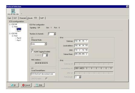
Repeat the same step for **Port 0** in the second ICG3 card, and enter an available IP address for the terminating ICG3 card in the **Local address** field. Click on **OK**.
