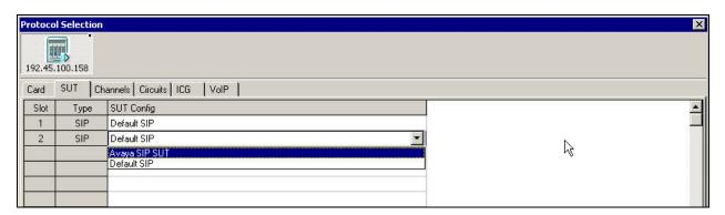
Maintain the defaults in the **Channels** and **Circuits** tabs. Should audio codec other than the default G.711 is desired, then this needs to be administered in the **Channels** tab. The following are the audio codec types that successfully interoperated between Abacus 5000 and Avaya Communication Manager during the compliance testing.
