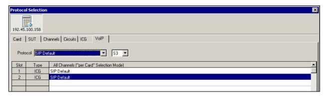
Click on the **Protocol** drop down list to optionally change the default value to "SIP180ringing". This will enable Abacus 5000 to send a ringing status for incoming SIP calls to the terminating ICG3 card, prior to the actual connection. Click on **OK** to submit the changes. The selection of "SIP 180ringing" for the second ICG3 card is optional, as the default value of "SIP Default" can work as well.
