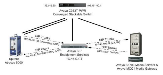
The compliance testing involved originating calls from the Abacus 5000 across a SIP trunk and terminating these same calls on the Abacus 5000 as SIP endpoints. The information from these Application Notes can easily be extended to other possible test scenarios such as:
