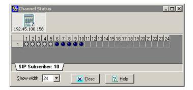
When the SIP calls have been established, then the color code for the corresponding channel will become green for the originating channels, and yellow for the terminating channels, as shown below. In this case, channels 1-5 are the originating channels, and channels 6-10 are the terminating channels.
