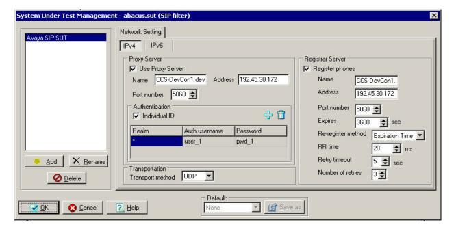
The **Protocol Selection** screen is displayed next. Click on the **SUT Config** field for the second ICG3 card, and select the newly created SUT from the drop down list. In this case, "Avaya SIP SUT". This enables the terminating ICG3 card to register the SIP endpoints with Avaya SES, using the SES proxy and registrar server information in the newly created SUT.
