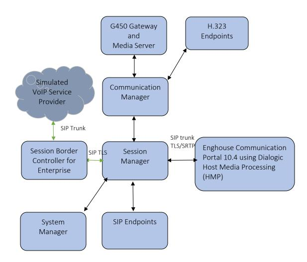
Figure 1: Test Configuration for Enghouse Interactive Communications Portal using Dialogic Host Media Processing (HMP) and the Avaya Platform.
