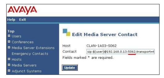
Figure 55: Fax / Modem Calls – Edit Media Server Contact Port Value
