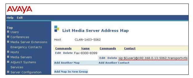
Figure 56: Fax / Modem Calls – Edit Media Server Contact Port Value
