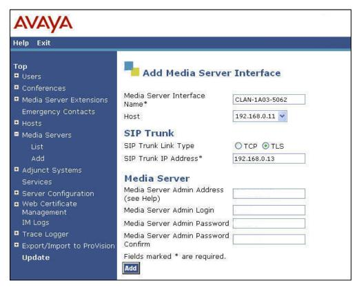
Figure 39: Add Media Server Interface for Fax / Modem Calling
