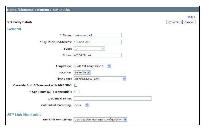
The following screen shows the addition of the 3800 Net-Net SBC. The **FQDN** or **IP Address** field is set to the IP address of the SBC's private network interface (see **Figure 1**). For the **Adaptation** field, select the Adaptation module previously defined for the SBC in **Section 6.4**. The **Location** field is set to **Belleville** which includes the subnet where the 3800 Net-Net SBC resides. Note that **SIP Trunk** was selected for **Type**.
