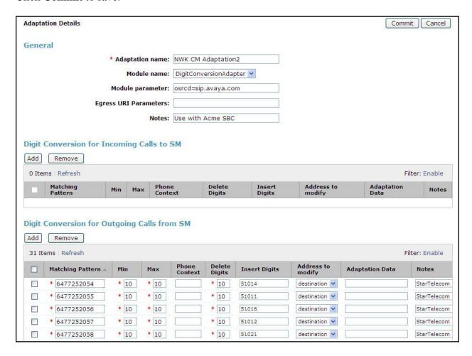
To create the Adaptation that will be applied to the 3800 Net-Net SBC SIP Entity, navigate to **Routing**  $\rightarrow$  **Adaptations** in the left-hand navigation pane and click on the **New** button in the right pane (not shown). In the new right pane that appears (shown below), fill in the following:
