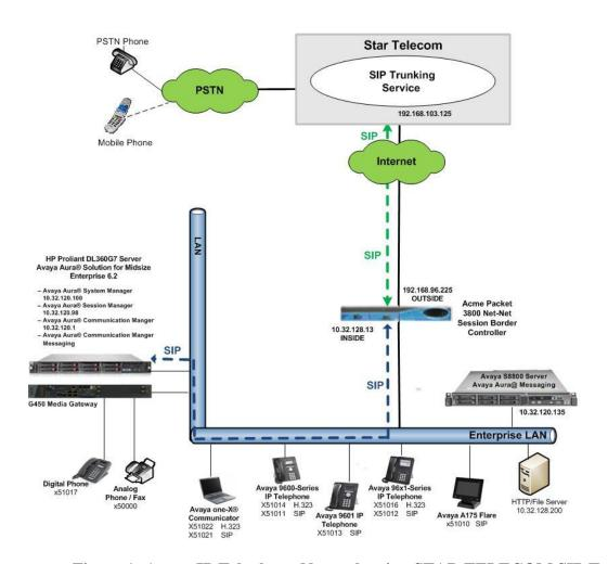
Figure 1: Avaya IP Telephony Network using STAR TELECOM SIP Trunking
