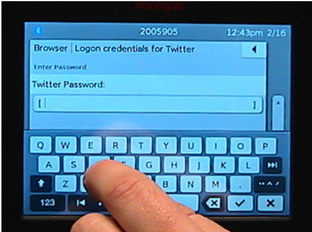
Figure 5-5: Avaya one-X 9670G deskphone showing touch-sensitive, on-screen keyboard
