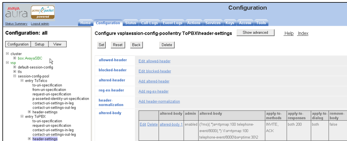
Figure 118: – Confirmation screen for the manipulation rule for Incoming Calls to Session Border Controller
