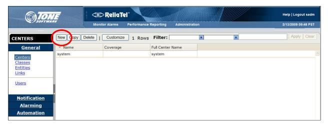
In the lower portion of the screen, select the **General** tab. Enter a descriptive **Name** for the center. Retain the default values in the remaining fields, and click **Apply**.
