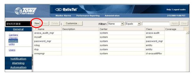
In the lower portion of the screen, select the **General** tab. Enter a descriptive **Name** and **Description** for the Avaya MSS. For **Center**, select the center name from **Section 6.2**, in this case "AvayaLab". For **Class**, select "cl-avayaAllPbx" from the drop-down list, as shown below. Click **Apply All**.
