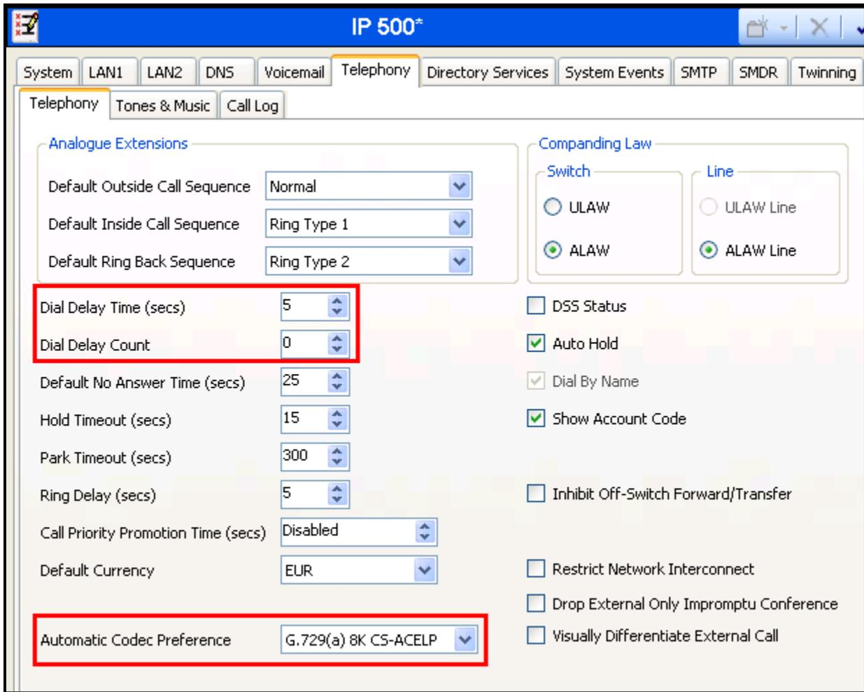
Figure 5: IP Office System: Telephony Tab
