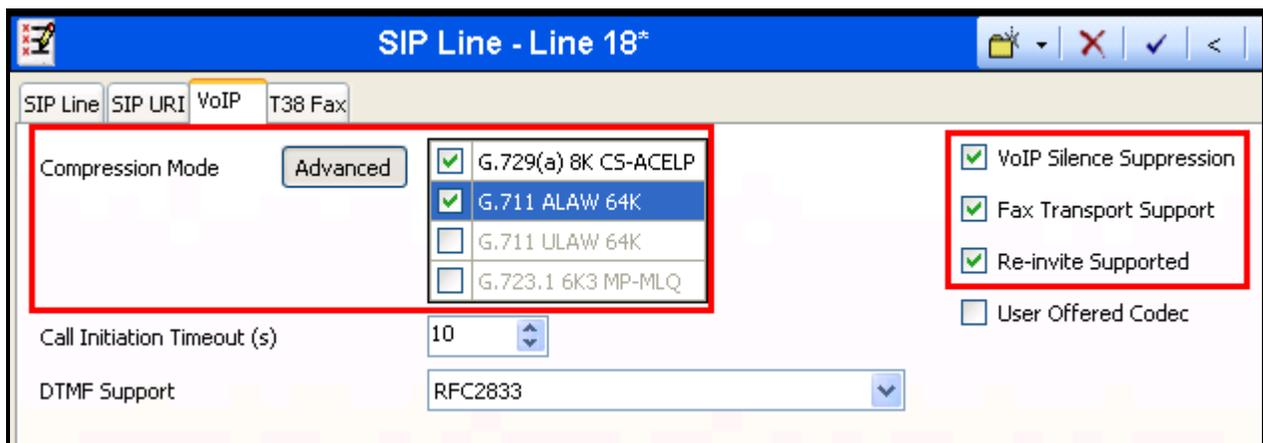
Figure 9: IP Office SIP Line: VoIP Tab
