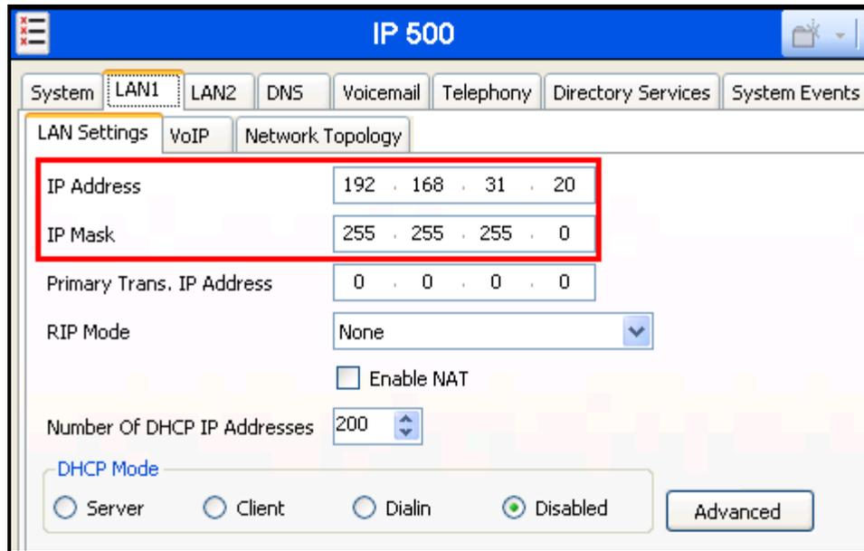
**Figure 4: IP Office System: LAN Settings Tab**
