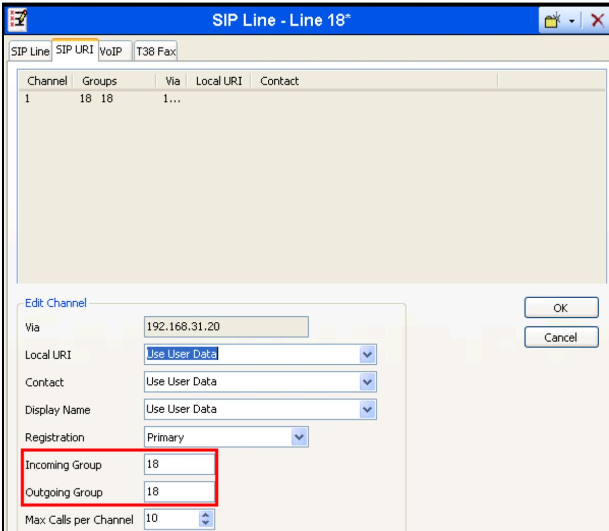
Figure 8: IP Office SIP Line: SIP URI Tab
