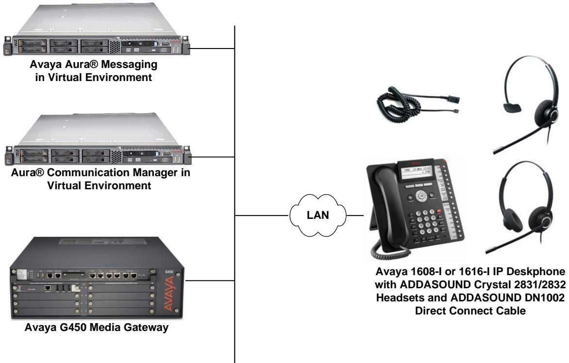
Figure 1: Avaya 1600 Series IP Deskphone with ADDASOUND Crystal 2831/2832 Headsets and DN1002 Direct Connect Cable
