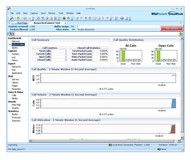
Select **Voice & Video > Calls** from the left pane. Verify that a call entry is displayed in the top pane for the active call. Note that the IP address 192.2.5.7 denotes the IP Media Processor board in the compliance testing. Select the call entry, and verify that the lower pane is updated with the call detail information. Double click on the call entry in the top pane to launch the Voice & Video Expert.
