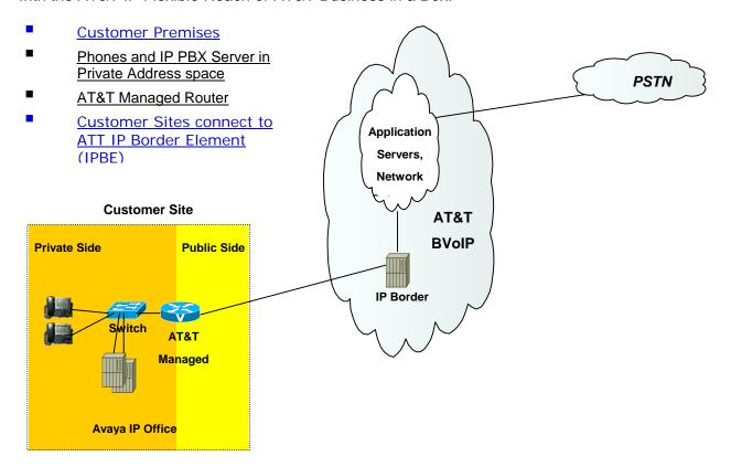
The diagram shows the IP Office system is deployed on the private side of the network and is linked to AT&T core network by an AT&T Managed router. This document contains configuration guidelines to the IP Office system only
