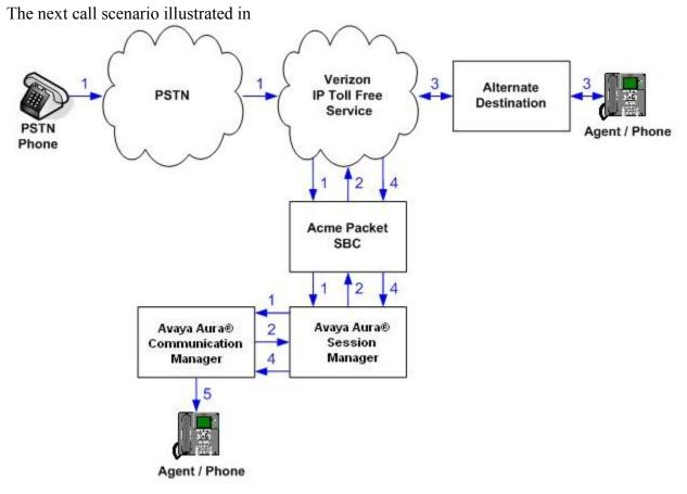
**Figure** 4 is similar to the previous call scenario, except that the redirection is unsuccessful due to the alternate destination being busy or otherwise unavailable. As a result, Communication Manager "takes the call back" and continues vector processing. For example, the call may route to an agent, phone, or announcement after unsuccessful NCR.
