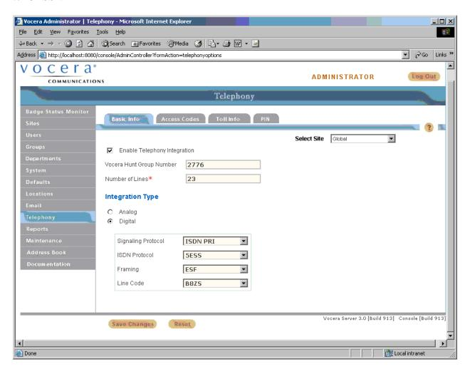
The following screen shows the configuration used when Vocera was connected to Avaya IP Office. The "Integration Type" was set to "Digital". The Vocera Telephony Server T1 was set to emulate the network side of the ISDN protocol, by setting the "ISDN Protocol" to "NT1".
