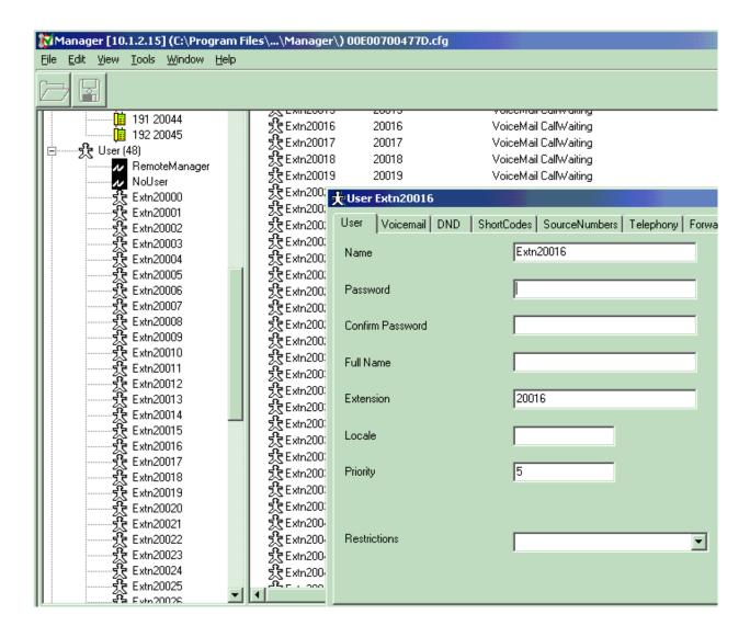
The extension configuration forms are under "Extension" in the "Configuration Tree". It is important to set the "Equipment Classification" to "IVR Port" for proper disconnect handling on the Vocera analog ports.
