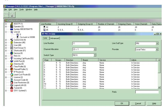
Avaya IP Office only supports the user side of the ISDN-PRI protocol, so the Vocera Telephony Server was set for the network side. The "Line Sub Type" was set to "PRI". The "Provider" was set to "Local Telco". The "Switch Type" was set for "5ESS", and 23 channels were allocated.
