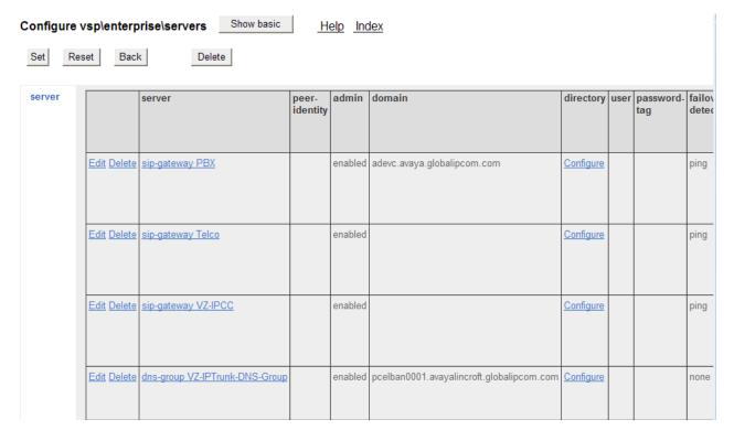
If desired, edit the newly created dns-group and assign appropriate attributes and policies that had been assigned to the "sip-gateway Telco" created by the installation wizard. For example, in the sample configuration, an "outbound-session-config-pool-entry" was assigned to the "sip-gateway Telco" created by the installation wizard. The procedure below assigns the same "outbound-
