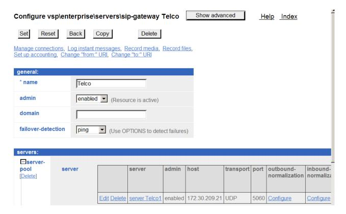
In the **port** field, enter the proper SIP signaling port used by the Verizon network. In the sample configuration, Verizon is expecting SIP signaling to UDP port 5071. as shown below. Click the **Set** button.
