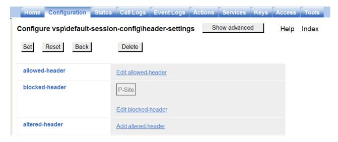
Similar procedures can be used to strip headers in a more specific session-config-pool. For example, to strip the P-Site header in the session-config-pool "To-Telco", navigate to vsp > session-config-pool > entry ToTelco > header-settings as shown below.
