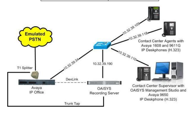
Figure 1: Compliance Testing Configuration
